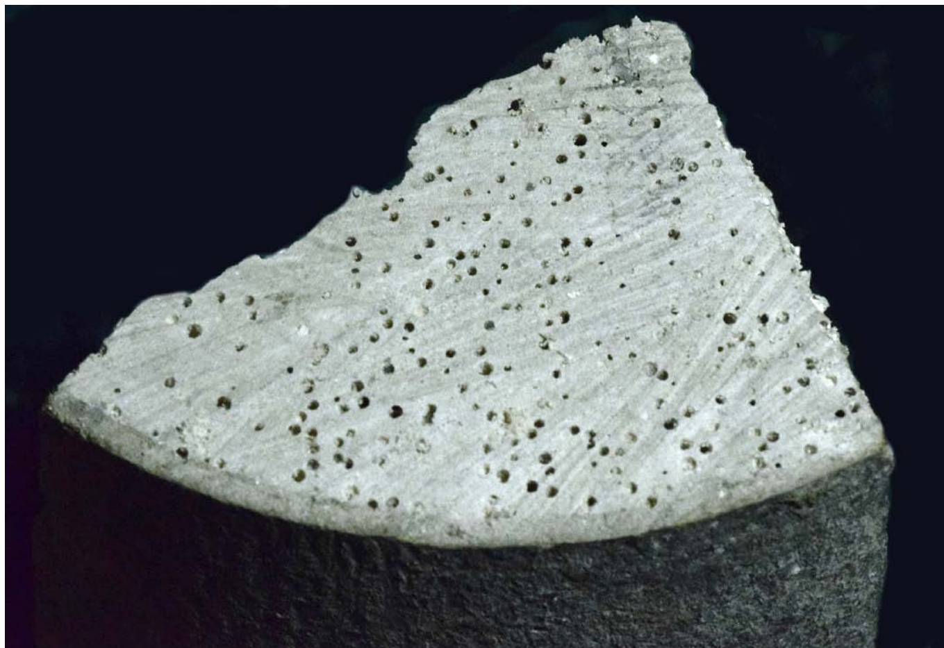
01. Segmented ash log, ex. wood store Pershore, Worcestershire, 7 January 2021, showing the density of Anobium punctatum galleries in transverse section.
